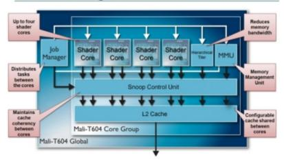
This dynamic load allocation, in turn, allows the host system to exert considerable control over the energy consumption of the core—vital to high-performance mobile use. But it also requires that the threads be light-weight. And that puts stress on the L2 cache, which must hold any state not local to the shader.
